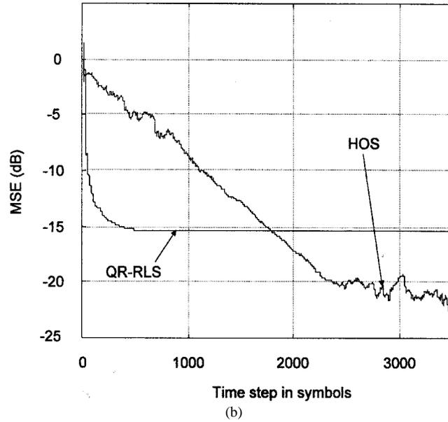
Fig. 6. MSE performance for the HOS (blind) algorithm and the QR-RLS (perfectly trained) filter. The delay interval for the three channels are (a) 0.15, 0.25, and 0.5 and (b) 0.15, 0.5, and 0.75.
