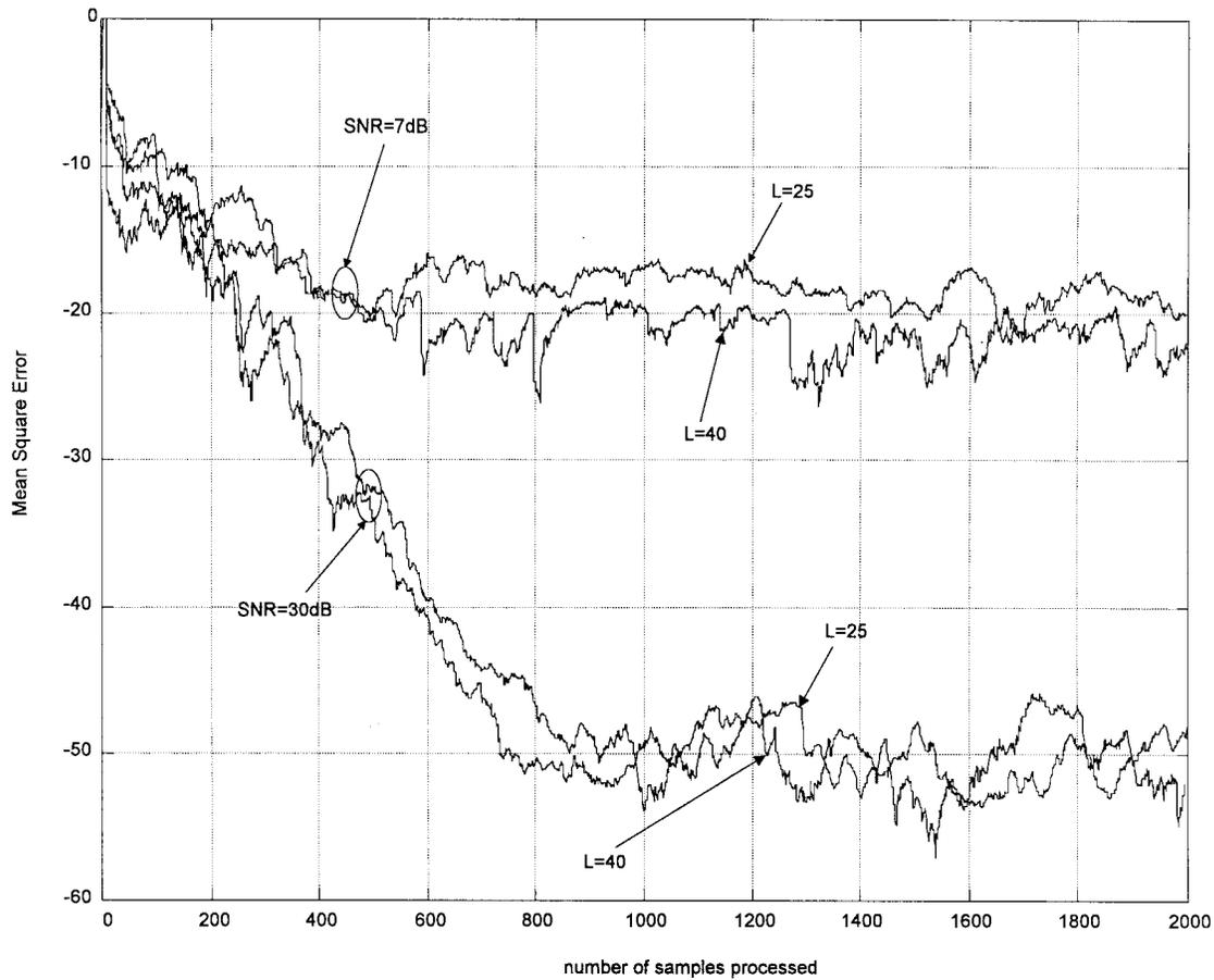
Fig. 5. Convergence process (same conditions as Fig. 4) for different SNR's on the first path—changing the length of the deconvolution baseband filters.
