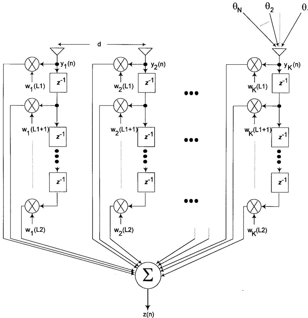
Fig. 2. Discrete-time model of the filtering section ( $K$  sensors and  $N$  paths).
