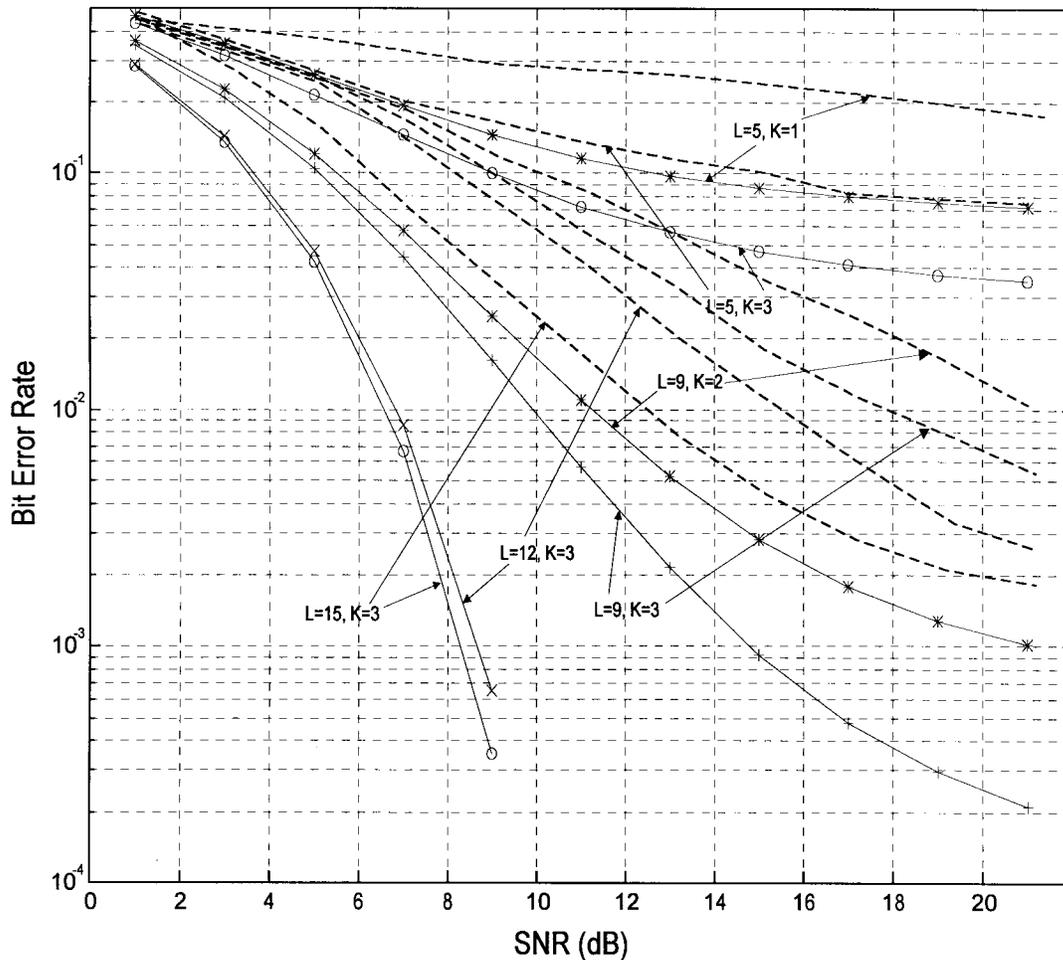
Fig. 9. Bit-error rate performance on a time-varying channel (the product maximum Doppler frequency-symbol period is equal to 0.0006) for different numbers of elements and weights. Delay intervals are 0.15, 0.25, and 0.35. The forgetting factor is 0.98. Solid curves are the performance of the HOS-based method, and dashed curves are the performance of the perfectly trained QR-RLS method.
