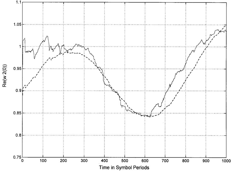
Fig. 8. Tracking performances of the QR approach with equal SNR's on all discrete channels (30 dB). The channel is varying, and the product maximum Doppler frequency-symbol period is equal to 0.0006. Delay intervals are 0.15, 0.35, and 0.75. The forgetting factor is equal to 0.97. The solid curve is the trace of the real part of the weight  $w(0)$  using the adaptive algorithm, and the dashed curve is the optimum performance.
