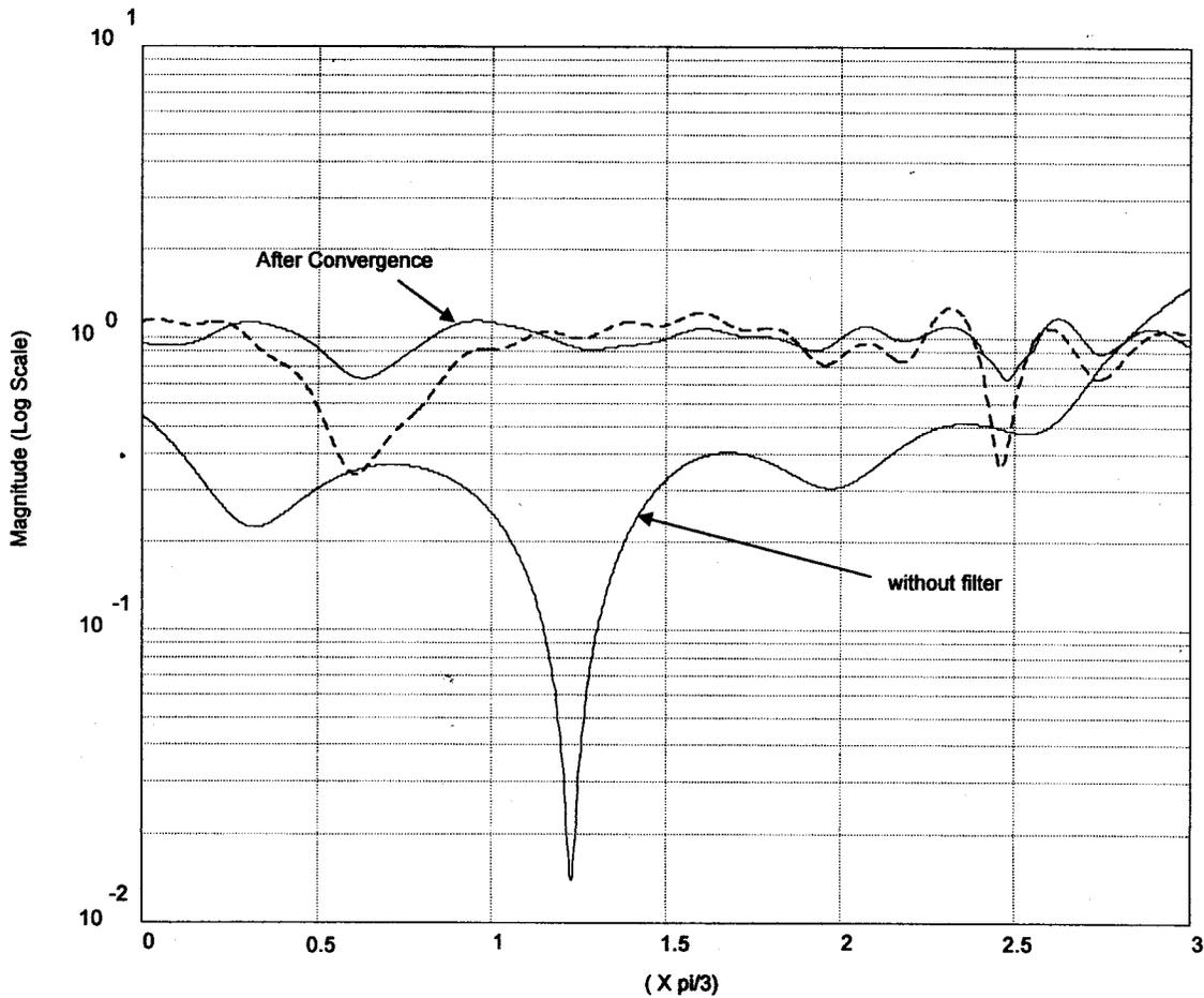
Fig. 7. Frequency response of the discrete-time system (channels-combining scheme) with no filter and after convergence (700 symbols) of the complex weights of the baseband filter (solid). Also, the response after 500 samples (dotted) is provided. The channel is in the same condition as Fig. 4.
