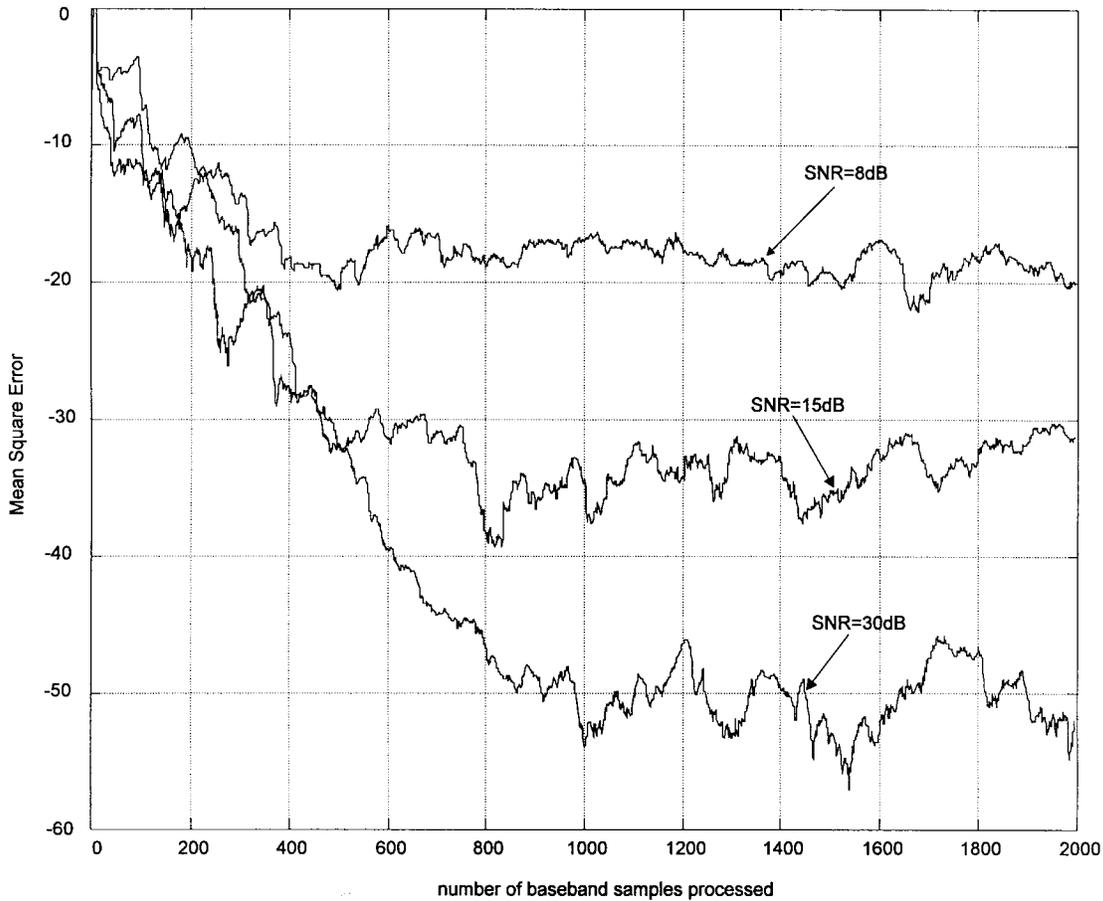
Fig. 4. Convergence process for SNR = 10 dB on the second and third paths and different SNR's on the first path. Delay intervals are 0.15, 0.25, and 0.35.
