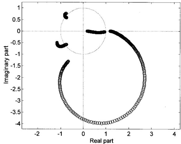
Fig. 3. Trajectory of the zeroes in the complex plane of the equivalent discrete-time model for the Rayleigh fading channel. These plots are representative of a fading event spanning 300 symbols. The speed of the mobile transmitter is 27 mi/h, and the delay interval  $D_i$  of the channel is 0.5. The NMP characteristic of the channel during most of the channel realizations is evident.
